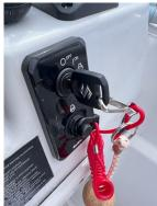
The next "key" is for the ignition and has a safety pin that has to be put in place to activate the ignition.
